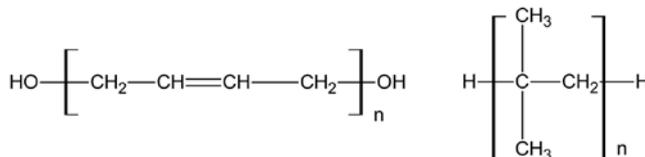
Fig. 1. Structure of HTPB (left) and PIB (right)
