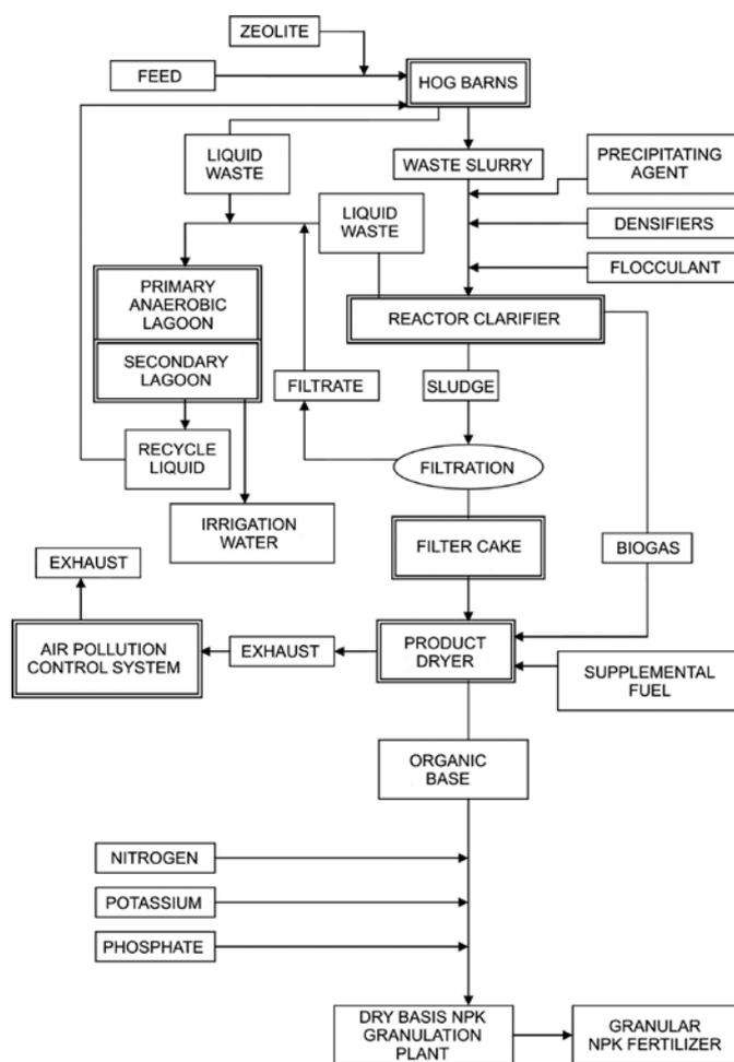
Fig. 1. Block diagram of pig manure processing methods [11]
