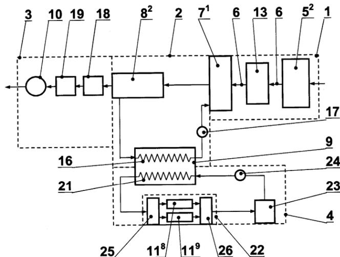
**Fig. 2. Flow diagram of a plant for generating and processing thermal energy from liquid manure, agricultural waste and food processing waste [27]**
