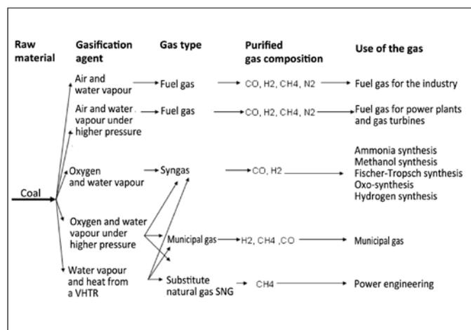
Fig. 3. Utilization of gas from the gasification process [4]
