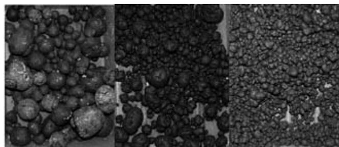
Fig. 5 Granulate produced from the coal slurry with the admixture of hydrated lime at an amount of: a) 1 % w/w of coal slurry b) 2 % w/w of coal slurry c) 3% w/w of coal slurry
