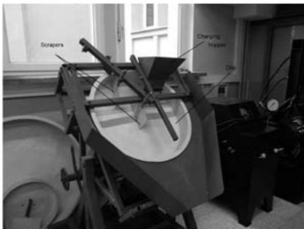
Fig. 6. Overall view of the granulating machine
