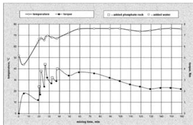
Fig. 6. Torque and temperature changes during production of USP pulp (test no. 1)
