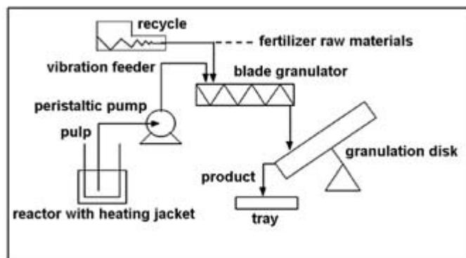
Fig. 8. Diagram of laboratory plant for fertilizer granulation
