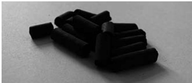
**Fig. 6. Pellets from post-hydrolysis lignocellulose with 20.6% moisture content**
