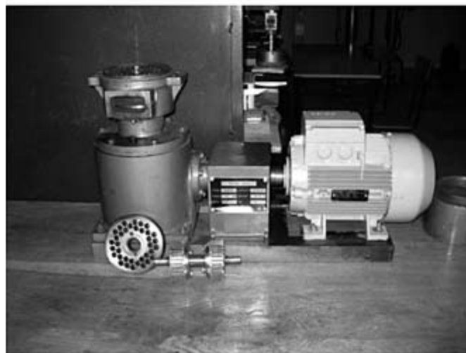
Fig. 11. Laboratory pelletizer with flat die
