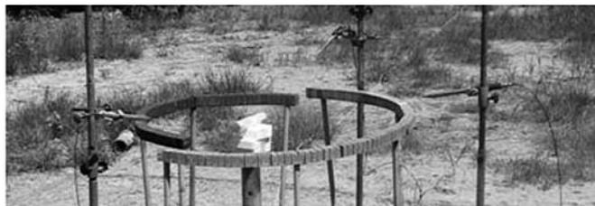
Photo 1. Test setup in Held's Method with piezoelectric sensors
