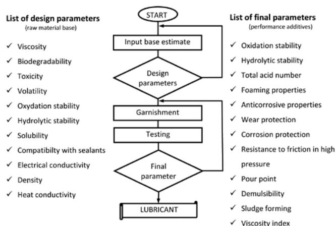
Fig. 7. Diagram of designing of lubricants [17]
