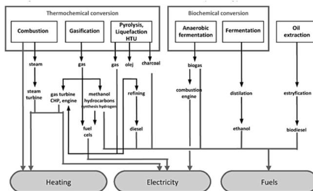
Fig. 1. Main technologies of conversion of biomass to secondary energy carriers [6]
