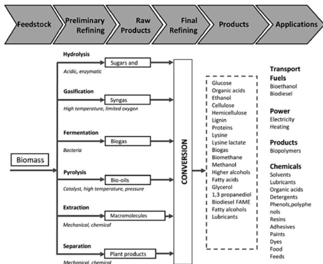
Fig.3. Biorefinery chart [9–12]
