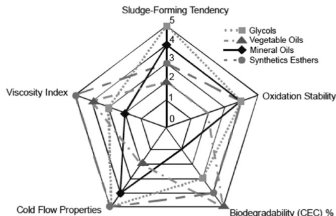
Fig. 8. Comparison of some properties of base bio-oil, mineral oil and synthetic ester [17]
