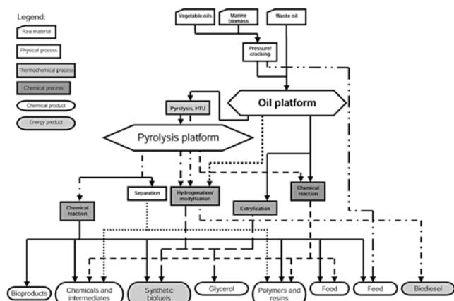
Fig. 4. Use of oil biomass in biorefineries [13]
